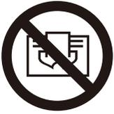
**Warning: this product shall be installed in the volume 2 only according the national wiring rules (For France NF C 15-100)**
