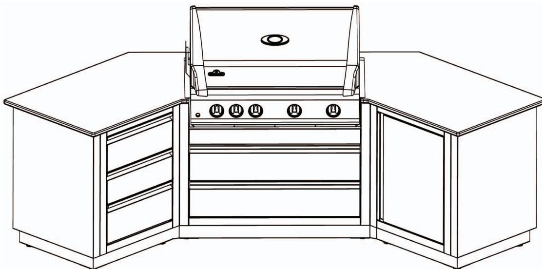
The above example is shown built as a stand alone island. Below, the dashed line represents the perimeter of the countertop (not supplied). The unit is angled by applying the IM-45T kit on either side of the unit which rotates the side cabinets at a 45° angle. Also shown is the IM-CEP, end panel, which creates a finished look to the ends of the assembled cabinets by covering the exposed knockouts and mounting holes.
