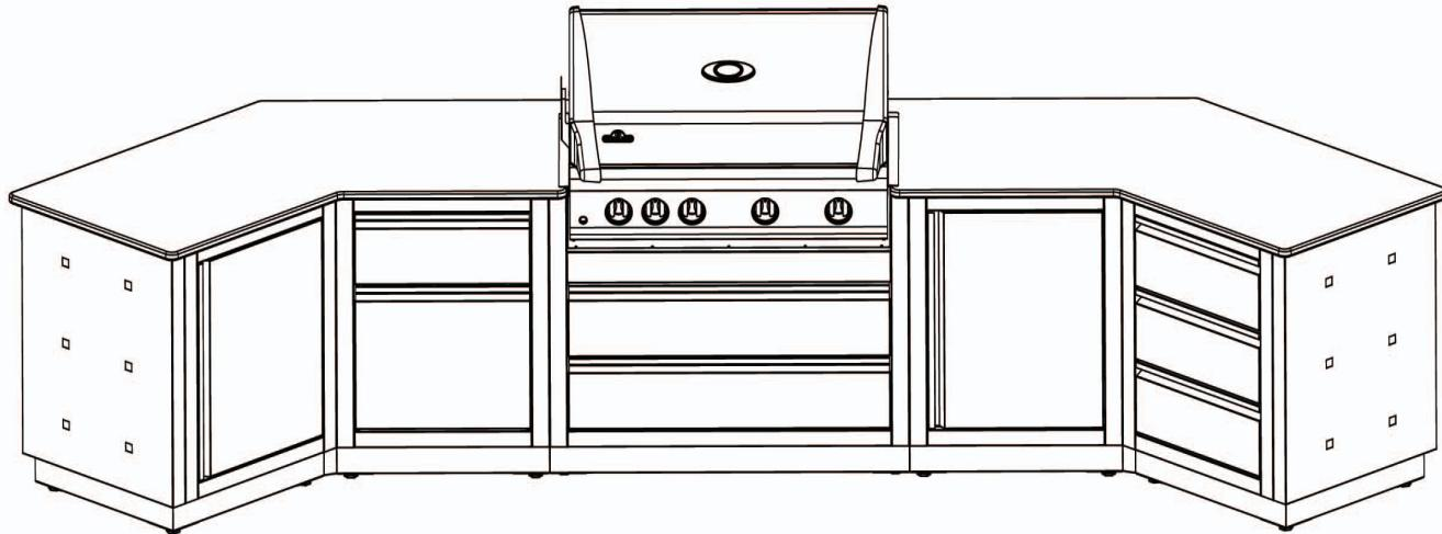
The above example is shown built as a stand alone island. Below, the dashed line represents the perimeter of the countertop (not supplied). The unit is angled by applying the IM-45T kit between the cabinets which rotates the side cabinets at a 45° angle. Also shown is the IM-CEP, end panel, which creates a finished look to the ends of the assembled cabinets by covering the exposed knockouts and mounting holes.
