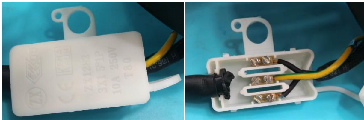
Photo 9: terminal block view for models LS-PPE01; LS-PE517; LS-PE518; LS-PPE01; 5777-P016; 5777-P018
