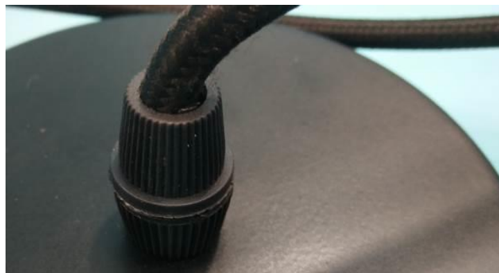
Photo 11: cord anchorage view for models LS-PE9006; LS-PE517; LS-PE518; LS-PPE01; 5777-P016; 5777-P018
