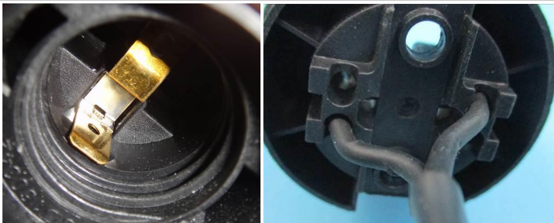
Photo 45: E27 lampholder and internal connection view for model 5777-P032
