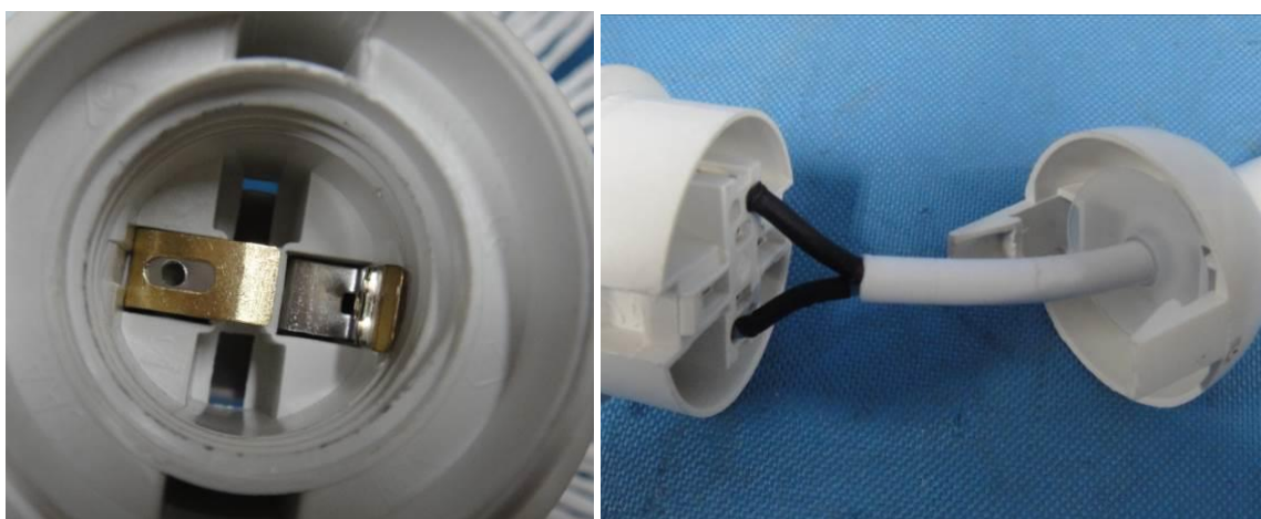
Photo 50: E27 lampholder and internal connection view for model 5777-P017
