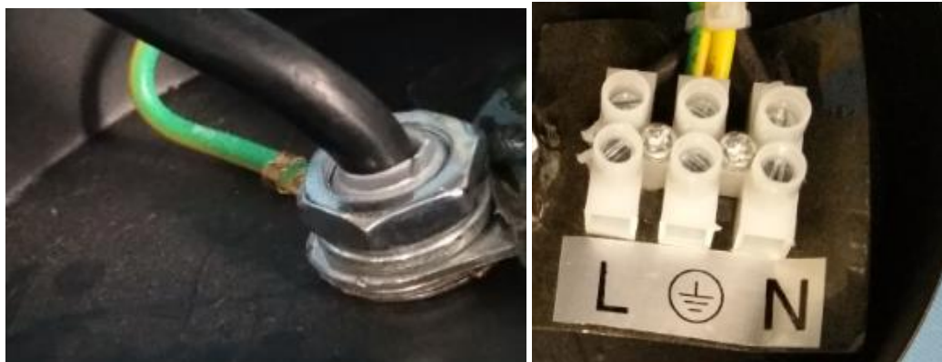
Photo 32: earthing connection and terminal block view for model LS-PE863
