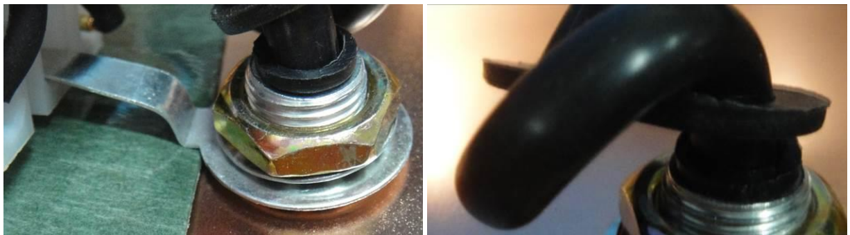
Photo 43: earthing connection and cord anchorage view for model 5777-P032
