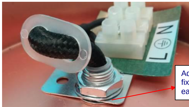
Photo 26: internal cord anchorage and earthing connection view for models LS-PE676A (TI-CP-0917); LS-PE0917A (TI-FCP-0917A); LS-PE0917B (TI-FCP-0917B)
