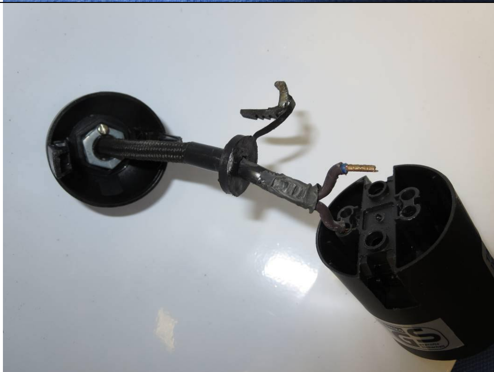
Mushroom shaped cord anchorage inside lampholder
