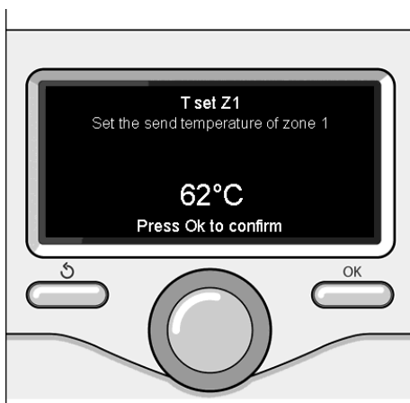
Change heating hot water temperature
