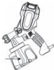
If you are going to be spraying in an upward direction, the angled end of the suction tube should be pointing toward the rear of the gun.
