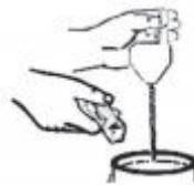
3. Hold the test cup up and measure the time in seconds until the liquid empties out. This time is referred to below as Runout Time.
