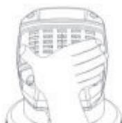
2. Remove the dirty filters and replace with new ones.
