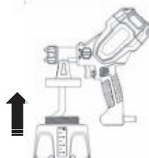
5. Attach the cup to the gun and plug in the sprayer.
