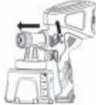
11. (a) Clean the rear of the spray gun with the appropriate cleaning solution.
