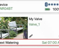
Once the programming is completed, the main valve dashboard should show the next watering schedule with the date and the hour.
