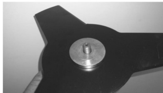
External disc washer disc fastened to secure the disc.
