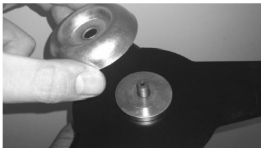
Placing the protective metal cup.
