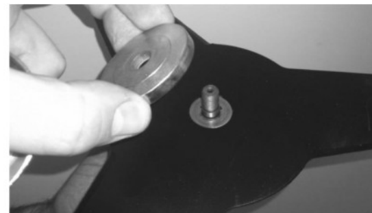
Attaching the outer locking washer with the part facing the disc.
