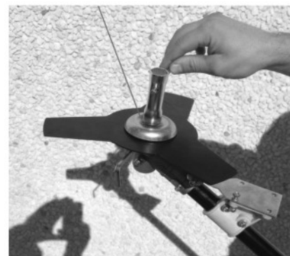
Locking nut to the left (counter clockwise)
