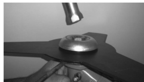
Nut tightening to secure the disc.
