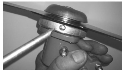
Attach the L-wrench to the side bore of the head to secure the disc's support shaft.
