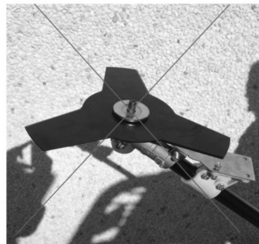
Disc locking washer incorrectly set.
