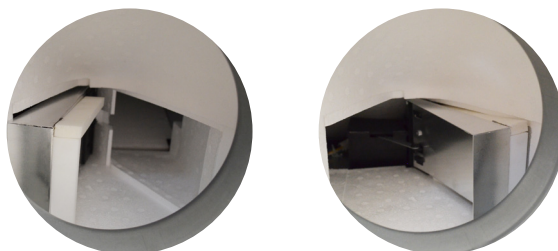
Fig. 13. Bypass is opened/ closed.
