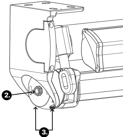
3. Turn the allen key by acting on the two inner studs with an allen key n°5, turn one or the other little by little, checking the direction of rotation to adjust the arm to the desired position. Once the position has been selected, tighten the screw in step 2 and fit the plastic covers.
