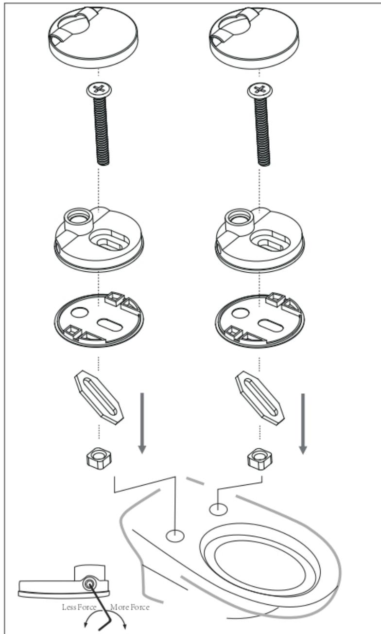
Just one or two turns, do not unscrew completely.
