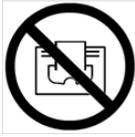
The heater must not be placed immediately under a socket outlet.
