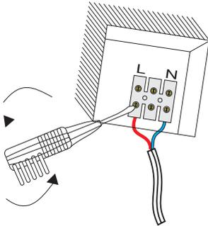
Before hanging the mirror, proceed to unscrew the box located on the mirror cable. In this, each of the cables coming from the light point of the wall will be hooked.
