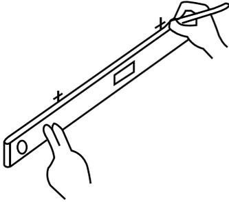
Measure the different distances corresponding to the height with respect to the sink and the screws to hold the mirror. Using a level, mark where the mirror hooks will be needed.
