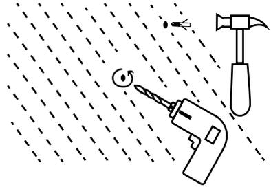
Drill the marked spots and place the dowels on the wall. Then place the hooks where the mirror will hang.
