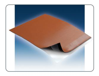
WAKAFLEX® a rollable multi layer laminate consisting of Polyisobuthylene (PIB) with aluminium rib mesh insert and butyl strips at the edges. Wakaflex is the practical approved universal product for professional abutments at chimneys, walls and other rising structures, obtainable in different colours, widths and lengths.
