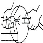
Always disconnect the air supply from the tool when the operation has been completed or suspended. When clearing a jammed fastener, moving to the different work area in order to adjust, disassemble or repair the tool.
