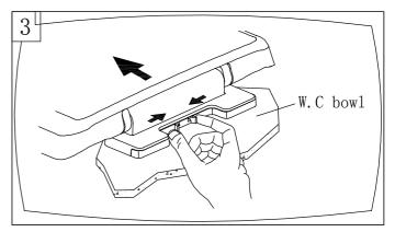
3. Disassemble: As shown in the figure, tightly pinch the fixture block at the direction of arrow, then take out the (7) at the direction of arrow.
