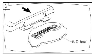
2. After finish steps shown in figure 1, install the ⑦ to the card slot of ⑤ at the direction of arrow. After install well, there will be a voice of "snap".
