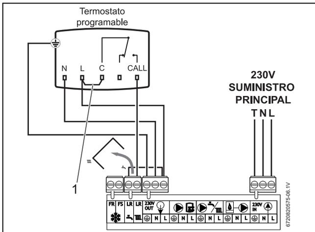
Fig. 61 Termostato programable
