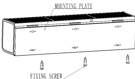
**2.2.2** Decide on the installation position and using the mounting bracket as a template, drill the necessary holes in the wall for correct installation.
