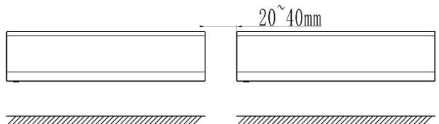
**2.5 Don't allow gaps between the unit and the wall.**
