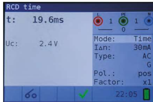
Figure 4-15: Example of trip-out time measurement results
