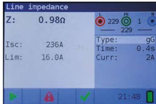
Figure 4 28: Example of line impedance measurement results
