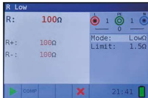
Figure 4 7: Examples of R Low resistance measurement results
