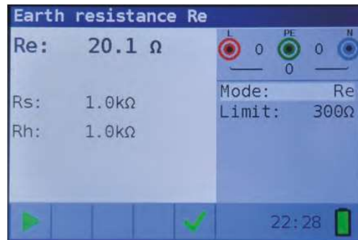
Figure 4 38: Example of resistance to earth measurement results
