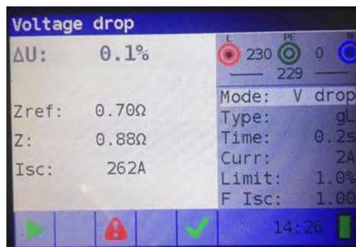
Figura 5 389: Example of voltage drop measurement results
