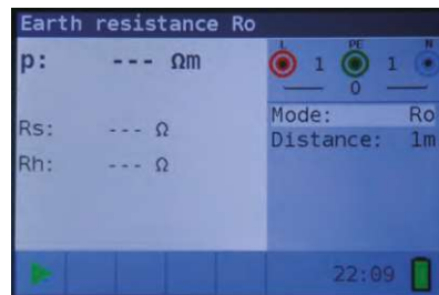
Figure 4 39: Specific Earth Resistance (Ro) measurement menu
