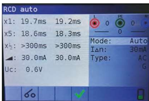
Figure 4 20: Step 8 RCD autotest results
