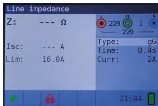
Figure 4 26: Line impedance measurement menu
