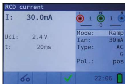
Figure 4 17: Example of trip-out current measurement result
