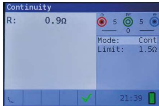
Figure 4 10: Example of Low current continuity measurement result
