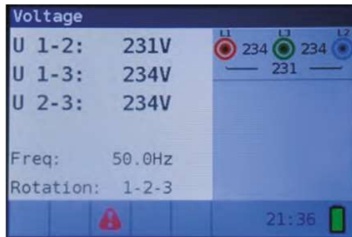
Figure 4 31: Example of phase sequence test result
