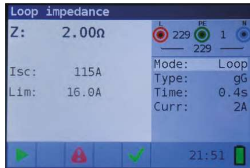
Figure 4 23: Example of loop impedance measurement results
