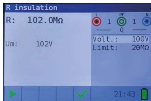
Figure 4 3: Example of insulation resistance measurement results
