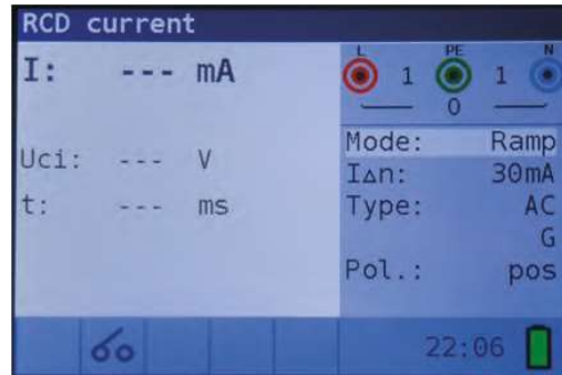
Figure 4 16: Trip-out current measurement menu
