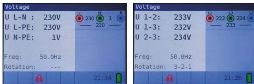
Figure 4 34: Examples of voltage and frequency measurements
