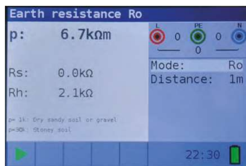
Figure 4 41: Example of specific earth resistance measurement results
