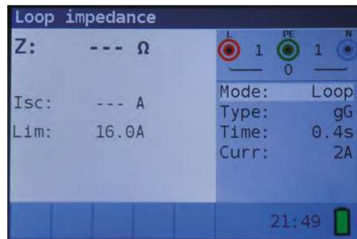
Figure 4 21: Loop impedance measurement menu
