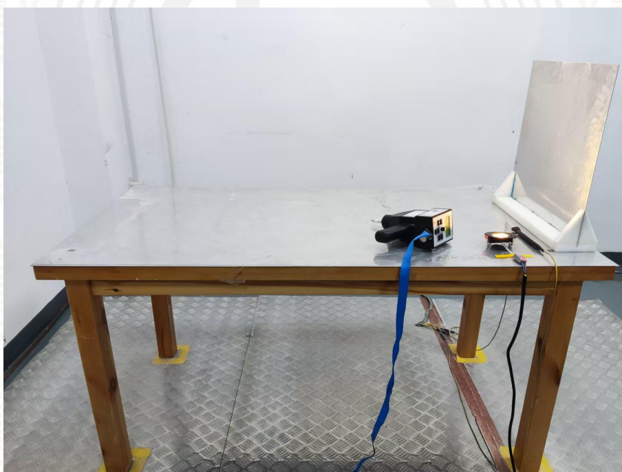
Figure 6: Electrostatic Discharge Test Setup
