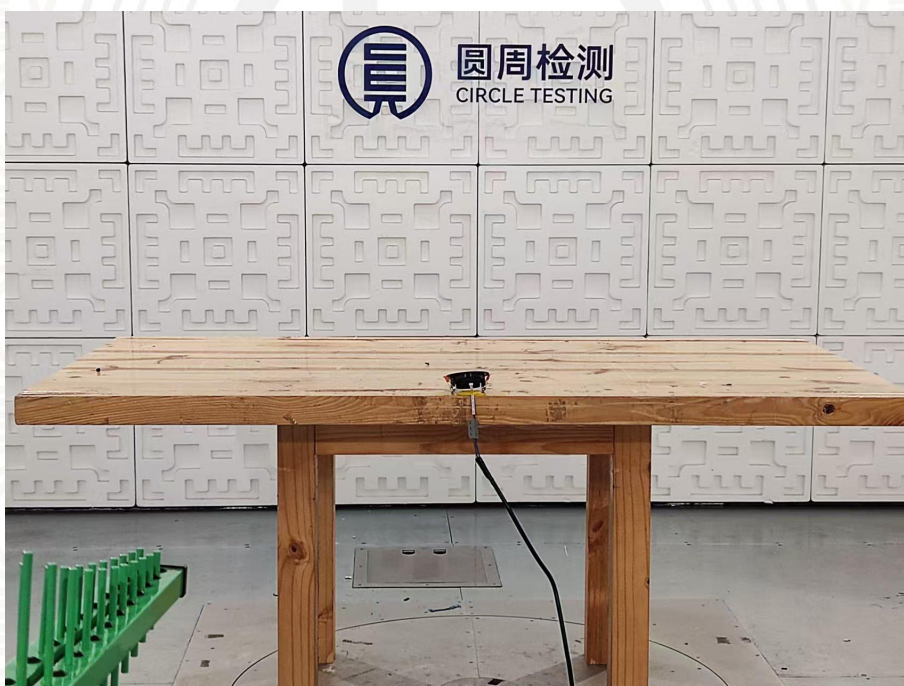
Figure 4: Radiated Emission Test Setup
