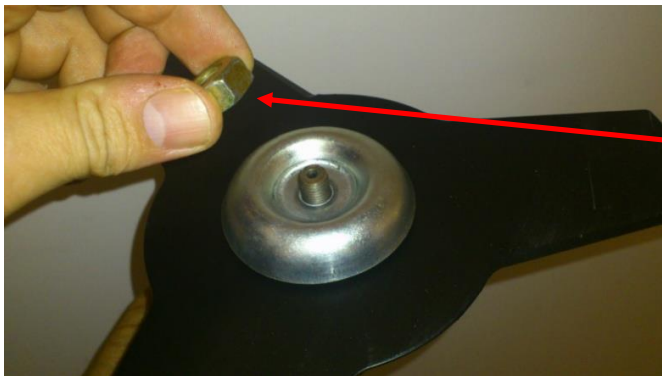
Placing the disc locking nut.
