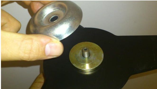
Placing the protective metal cup.
