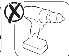
Do not screw the terminal to the mounting bracket using a screwdriver.
